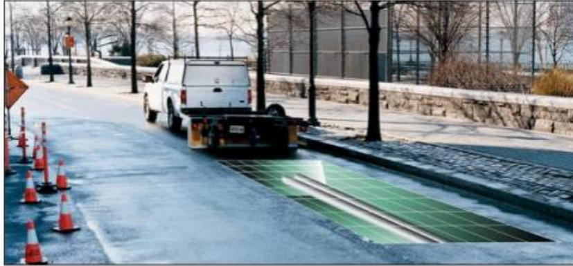
The Computer-Aided Radar Tomography Imaging System, in development, creates three-dimensional images of underground structures.
