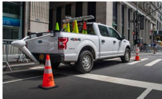
Along with scanning the entire service area for contact voltage (stray voltage) on a schedule, our trucks conduct scans before large public events
