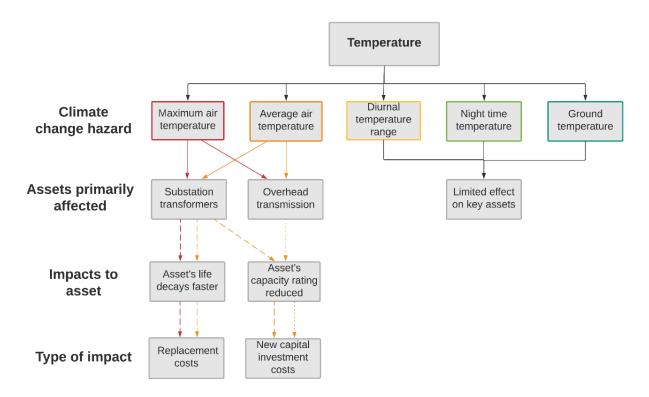
Figure 18 Temperature-related impacts on Con Edison's electric system
