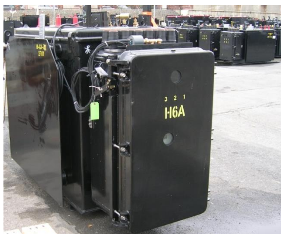
Figure 1: Network Transformer and Protector
